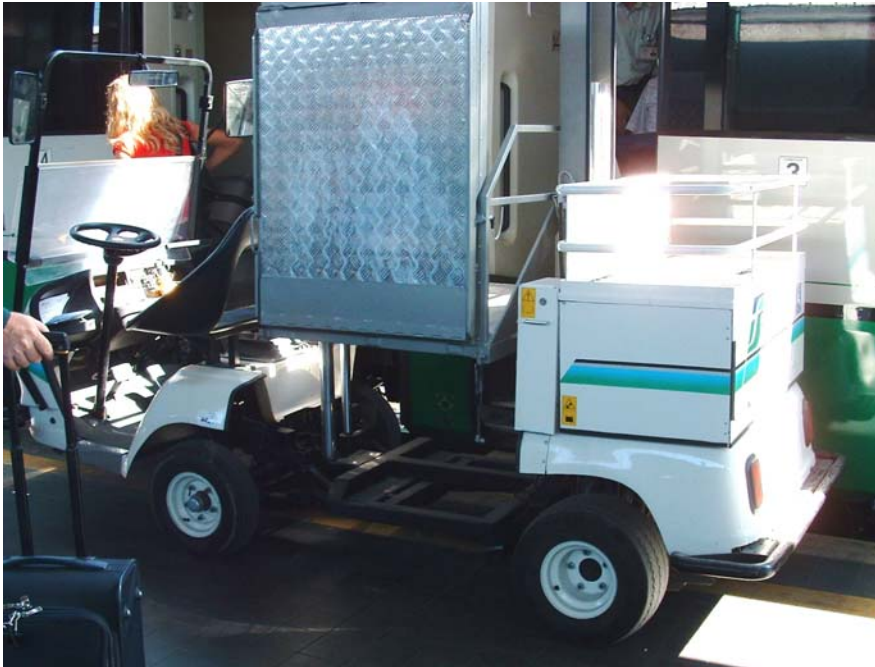
Photo 15. Trenitalia wheelchair lift for rail passengers
