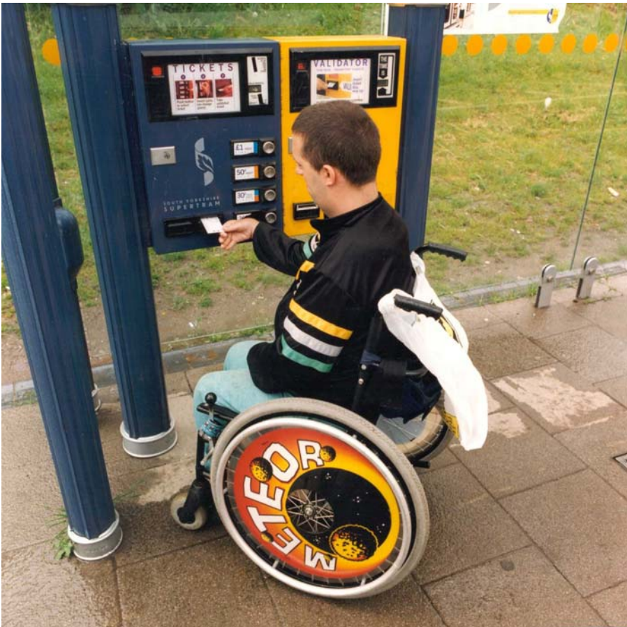
Photo 12. All operable parts of ticket machines must be reachable by wheelchair users
