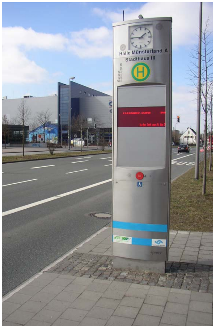
Photo 2. Dynamic information can be given audibly by this Passenger Information System in Munster
