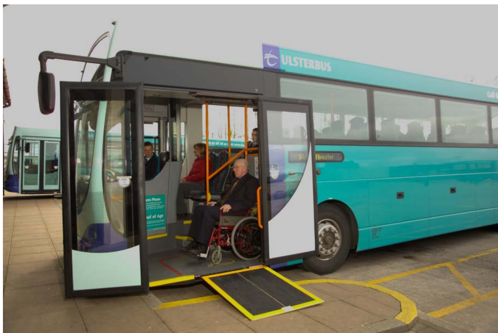
Photo 21. High-floor coach with ramp access to low-floor area
