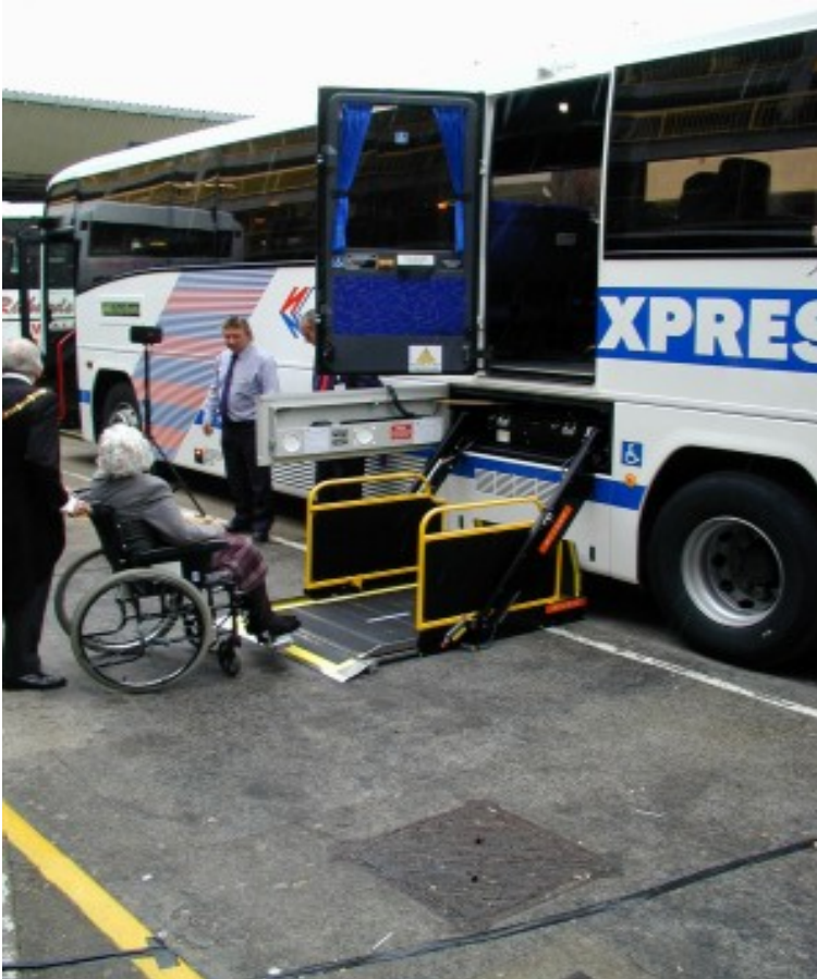
Photo 20. Access onto a high-floor coach is possible with an on-board lift
