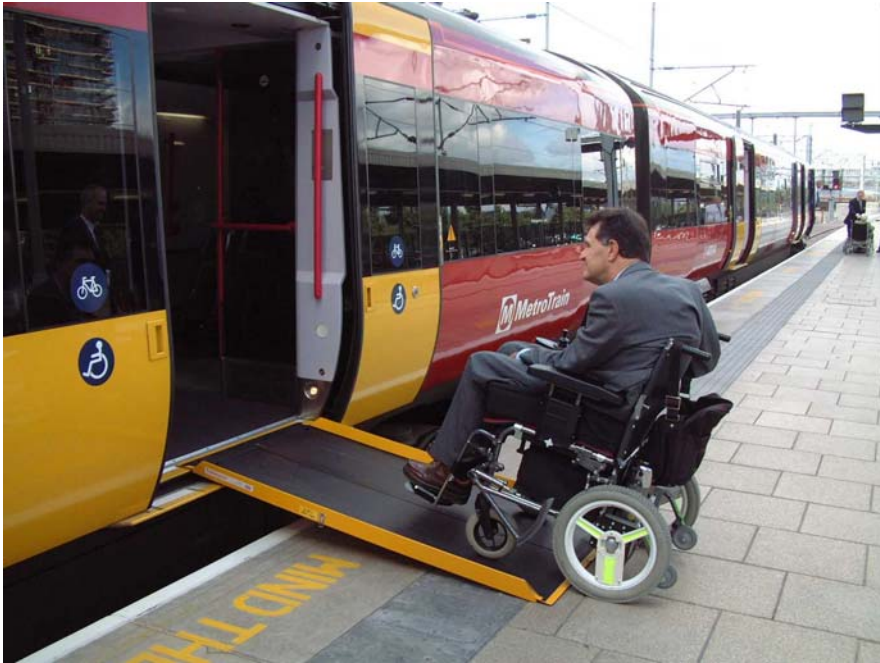
Photo 14. Direct train/platform access for wheelchair users
