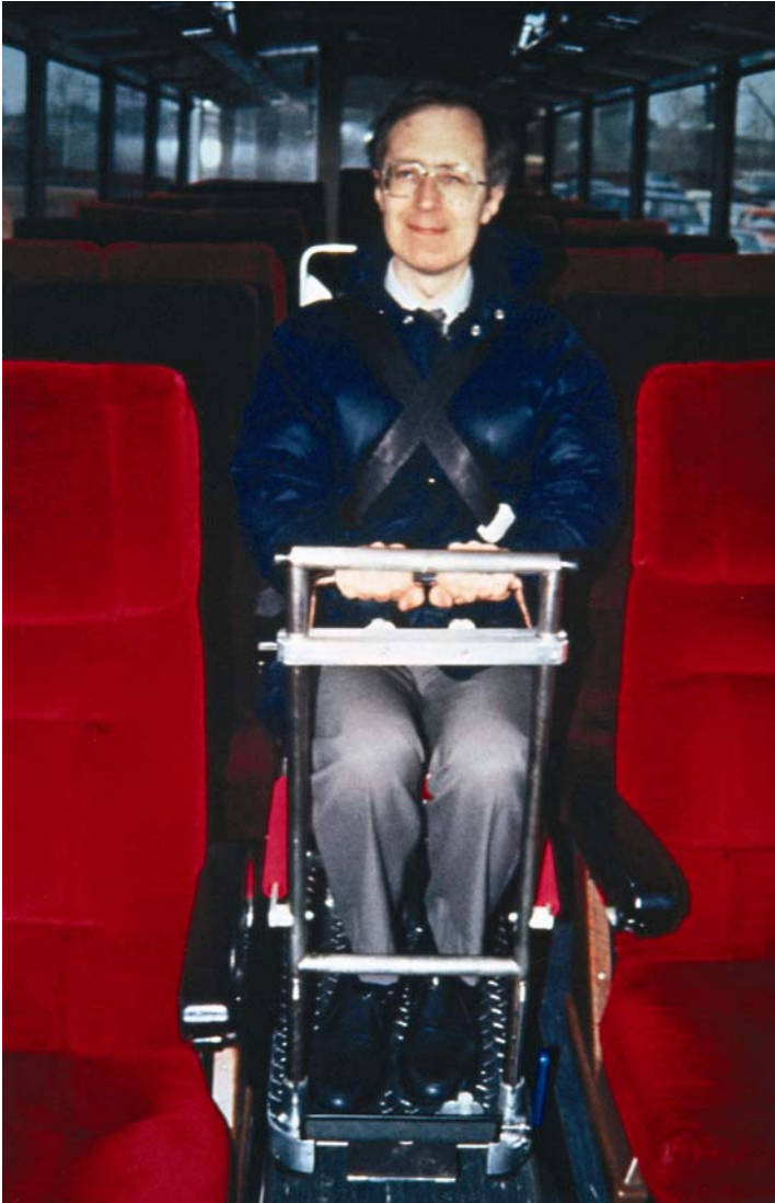
Photo 24. Specially designed wheelchairs can be used to assist passengers on vehicles with narrow gangways, including aircraft
