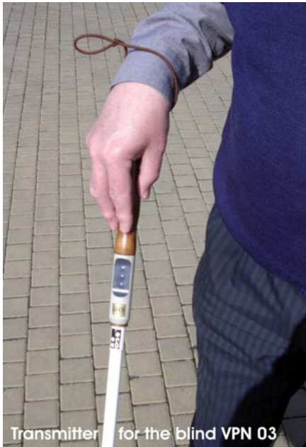
Photo 10. The Apex transmitter signals intention to board vehicle
