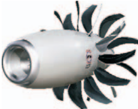
Figure 7.7 ▶ Open rotor engine design
