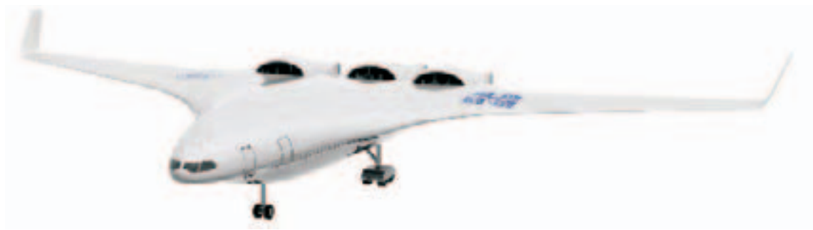
Figure 7.8 ▶ Blended wing body – SAX-40 design
