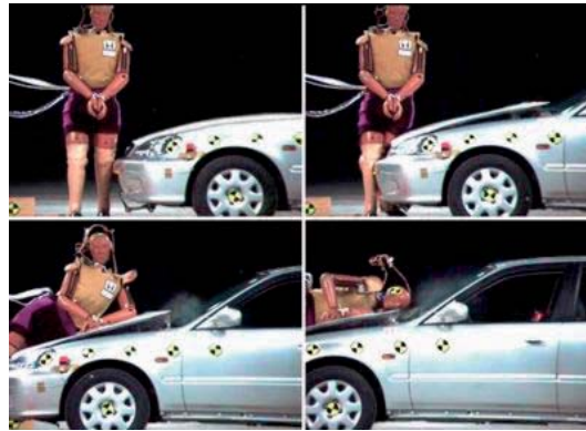
Figure 6.21. Innovative vehicle design: Bonnet airbag system
