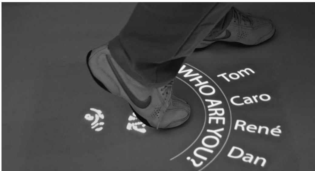
Figure 2.13. The Multitoe project: touch-sensitive floors
