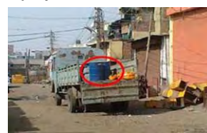
Source pencils transported in a lead container for proper disposal
