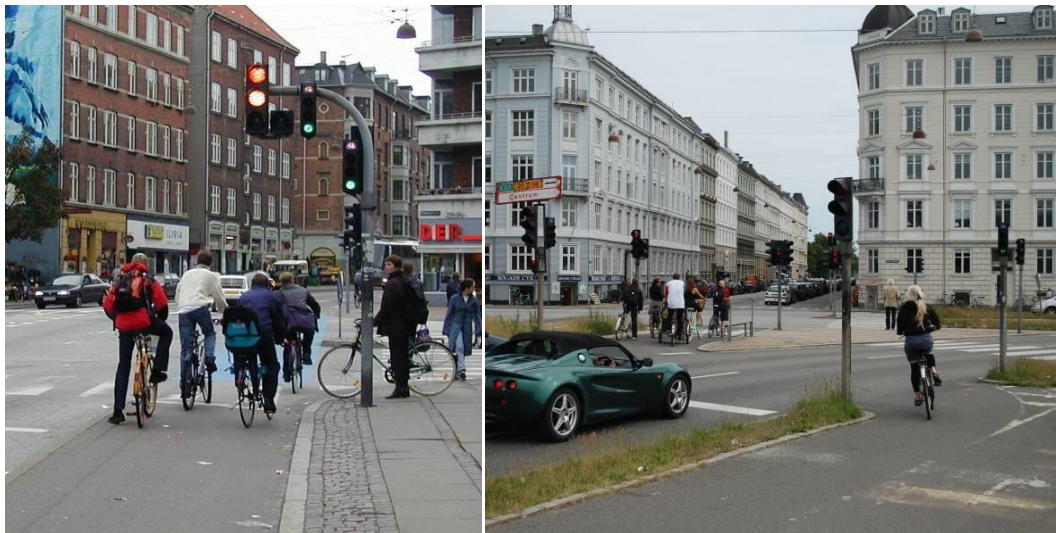
Figure 5.31 Bicycle-specific traffic signal phases
