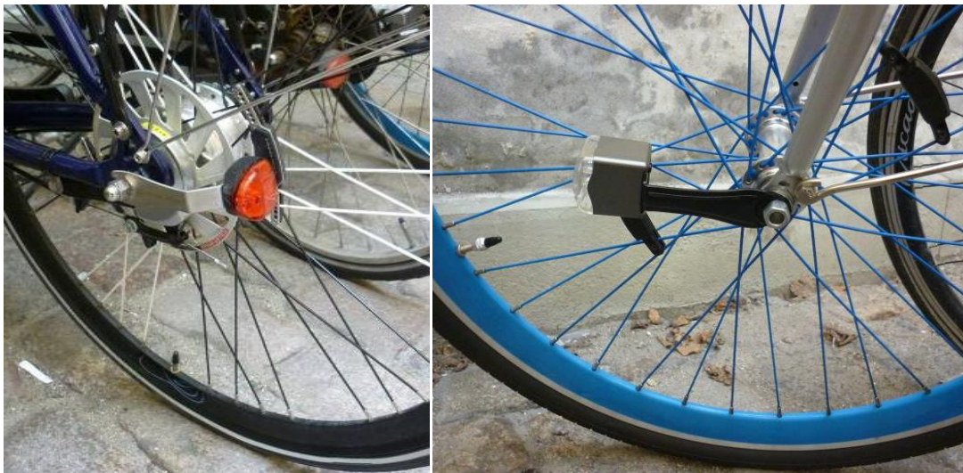
Figure 5.3 Tail and front lights (from two different manufacturers) powered by magnetic induction.
