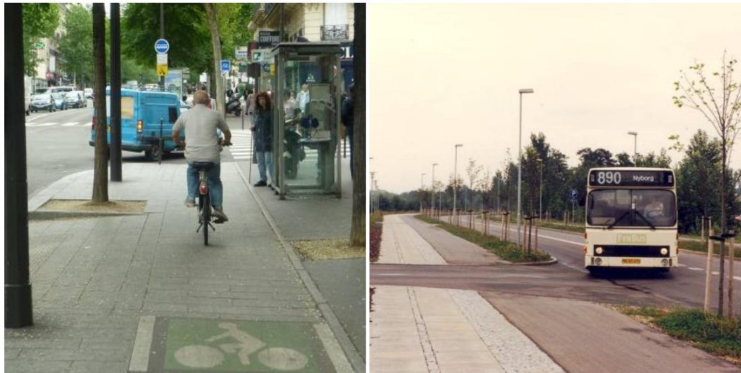
Figure 5.15 Some bicycle track designs (verges with trees, lamp posts etc.) may “hide” bicyclists from turning cars
