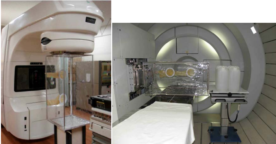
Figure 1: Irradiation set-up for activation of air for the electron accelerator (left) and air and water for the proton accelerator (right)
