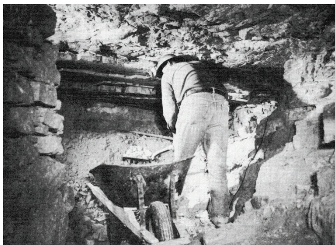
Figure 2.2. Hand loading ore onto a wheelbarrow in a small mine on the Colorado Plateau in the mid-1950s (Dare et al., 1955)
