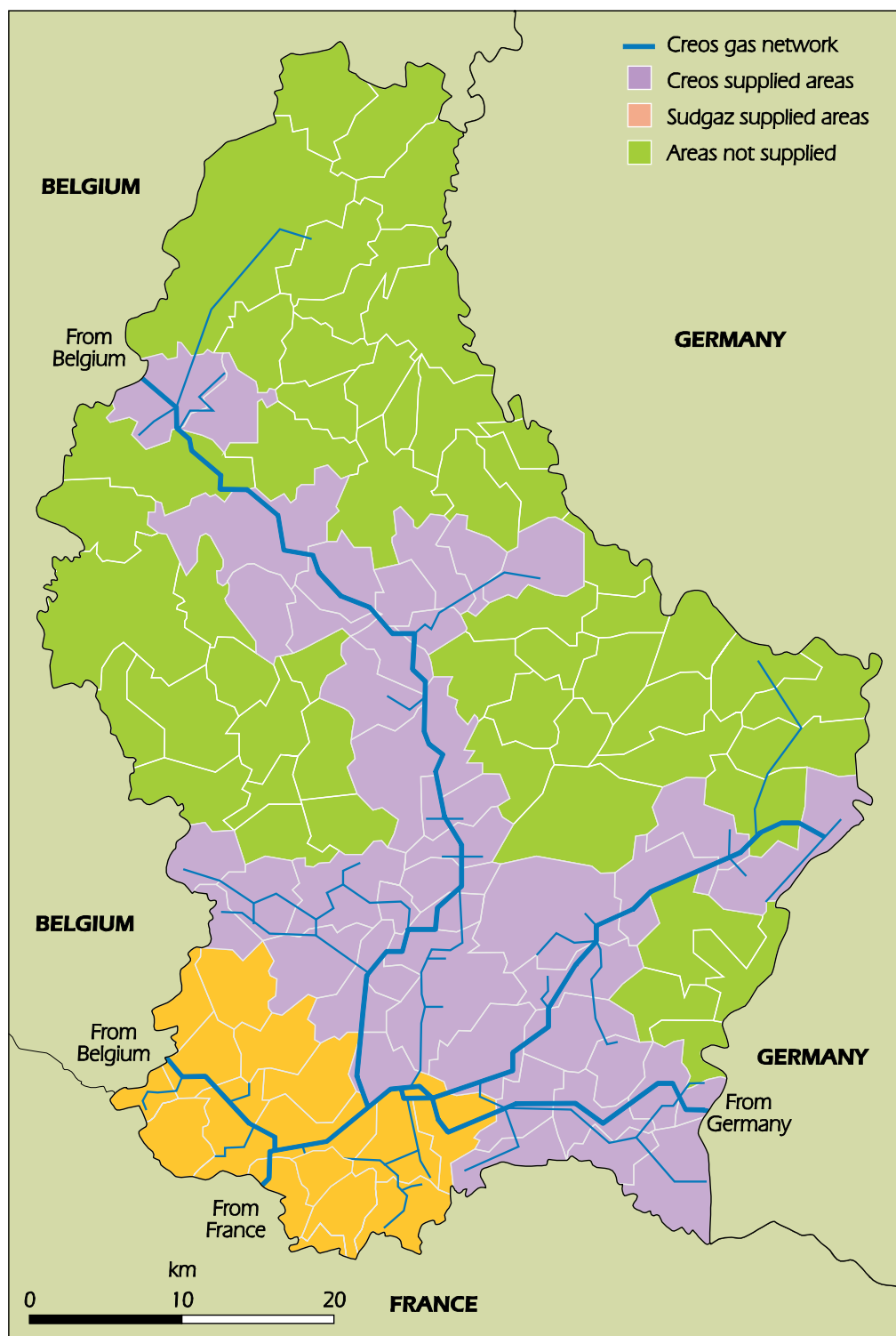
Figure 7.2 The natural gas network of Luxembourg, 2014
