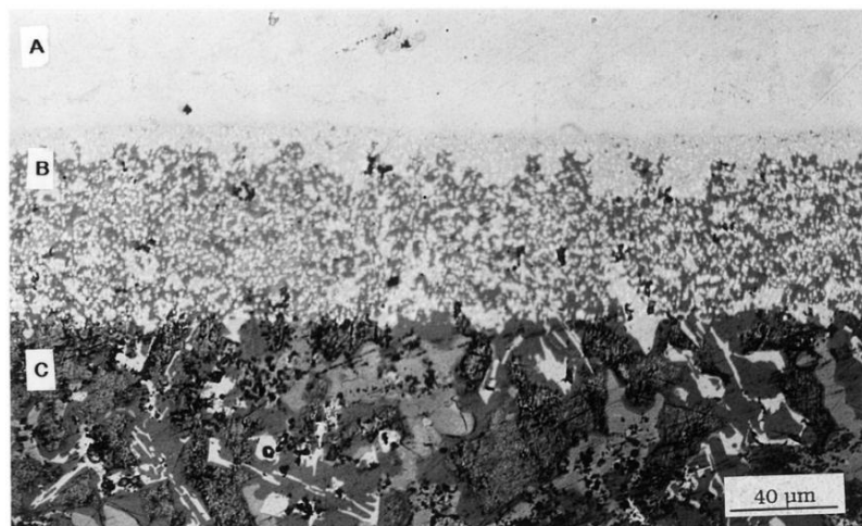
Figure 2.7: Reaction layer formed at REMAAL/15-15Ti interface [33]
