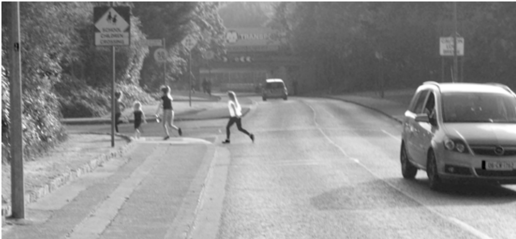
Figure 3.7. Urban road with inadequate pedestrian provision: a design focused on keeping traffic moving rather than encouraging walking
