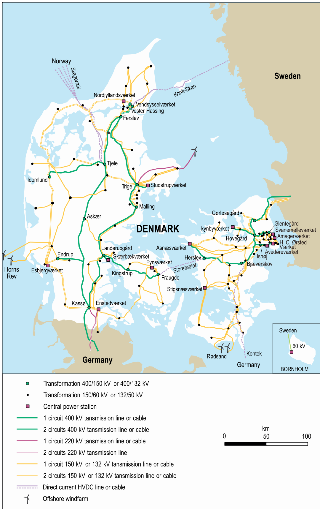
Figure 5.7 The Danish electricity transmission system
