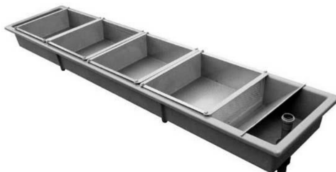
Figure 3.10. Standard hatching trough that may be used for Atlantic salmon egg to first feeding fry stage
