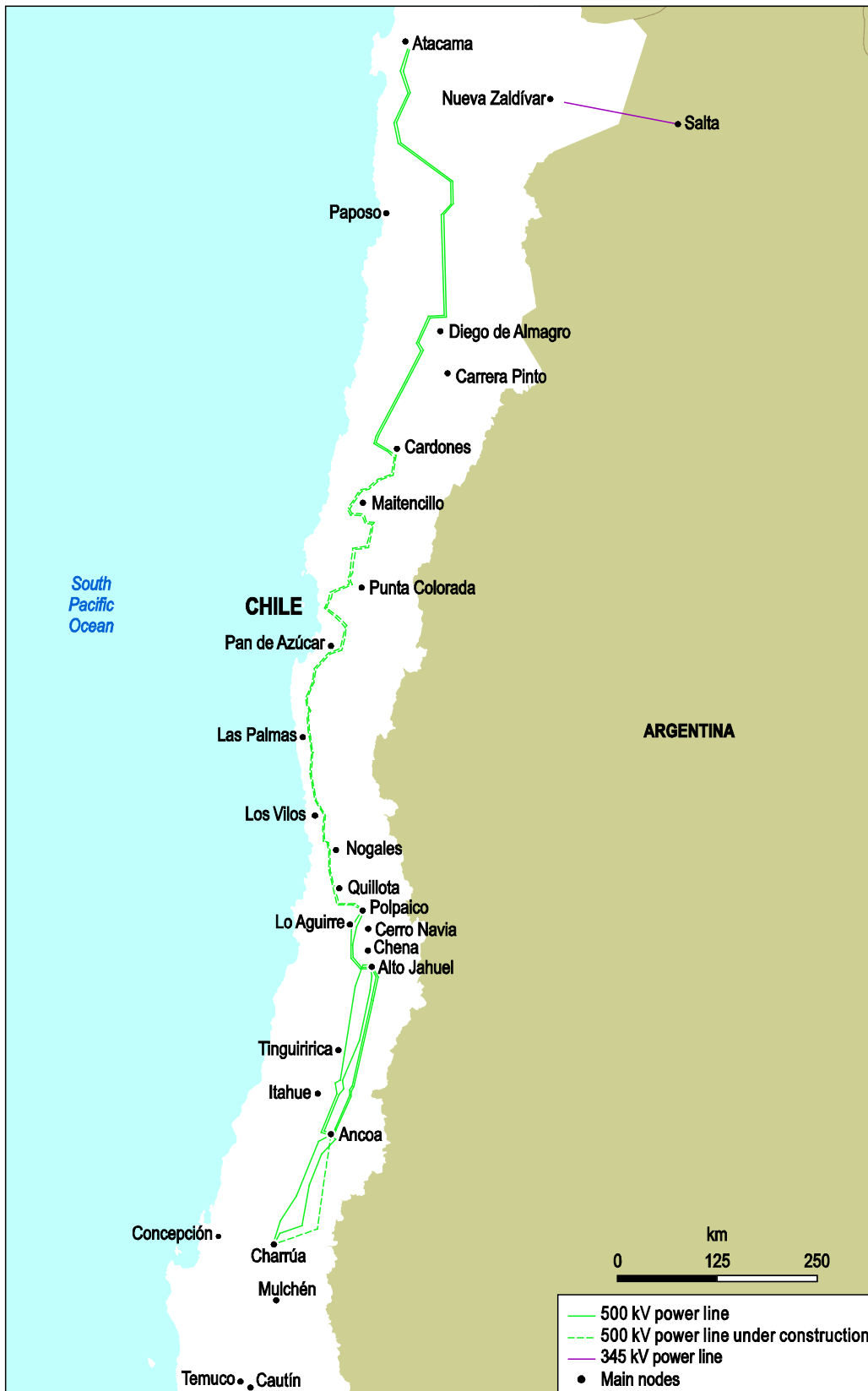
Figure 5.8 Map of the interconnected high-voltage electricity grid, end 2017
