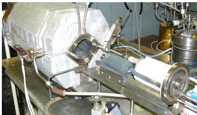
Figure 2.6. “Mini Khrust” pilot set-up (heater, ampoule for spent nuclear fuel and cork are observed)
