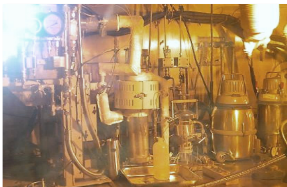
(a) Sintering off-gas trapping system
