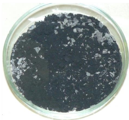
Figure 2.9. Voloxidised uranium dioxide nuclear fuel
