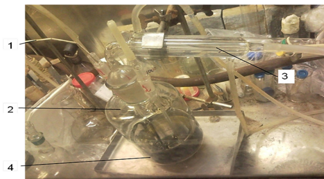
Figure 2.36. The laboratory facility for actinide melting showing 1 – a thermocouple in a glass pocket, 2 – an evaporator, 3 – a direct condenser and 4 – a solution of actinide nitrates
