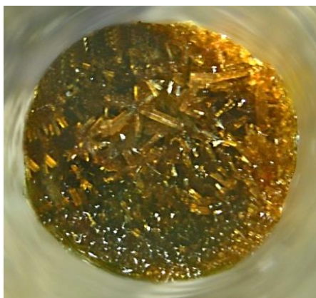
Figure 2.42. Crystals (U,Pu)O_2(NO_3)_2 \cdot 6H_2O with an increased content of plutonium
