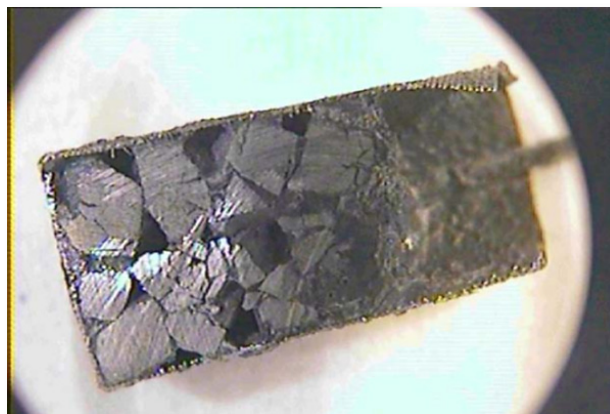
Figure 2.110. Reduced fuel particles of irradiated MOX fuel particles (43 GWd/tHM); section of cut basket
