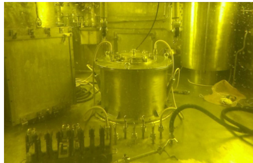
Figure 2.122. Zn distillation unit for clad material separation
