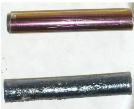
Fraction of non-irradiated fuel element (1) and sample after processing with the "mini Khrust" set-up (2)
