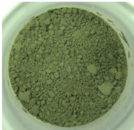
Figure 2.33. Image of the uranium oxide sample after denitration
