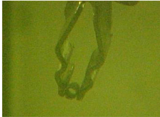
Figure 2.120. Empty cladding after anodic dissolution of nitride SNF in chloride melt
