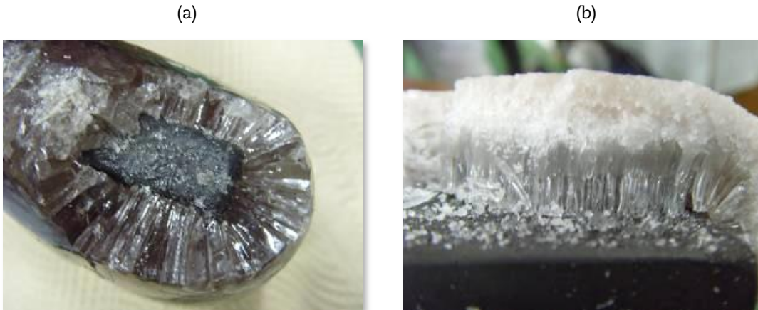
Figure 2.128. A crystal formed at the surface of the crystalliser
