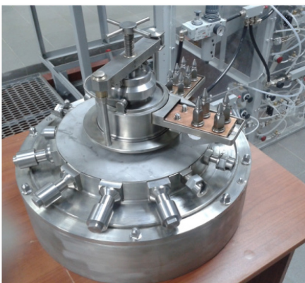
Figure 2.123. Electrorefiner up to 2000 A on cold test facility
