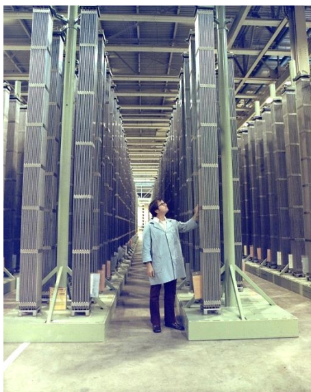
Figure 2.2. Westinghouse PWR fuel assembly
