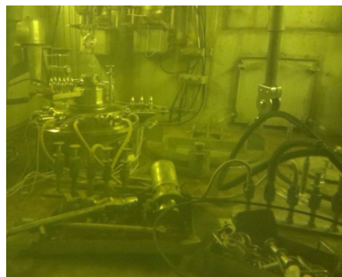
Figure 2.124. Electrorefiner in hot cell during test with real SNF
