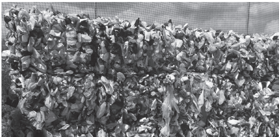
Figure 5.4. Mixed colour HDPE plastic bottles, baled ready for sale as a “sorted waste plastic”
