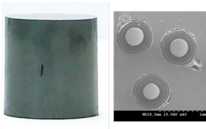
Figure 18.5. Optical photo and SEM microstructure of PBAT fuel pellet fabricated by pressure-less sintering process (by KepcoNF)
