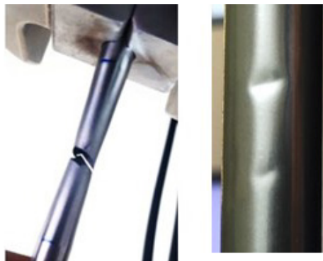
Figure 12.1. PM Mo tube after tensile test and local denting test at room temperature
