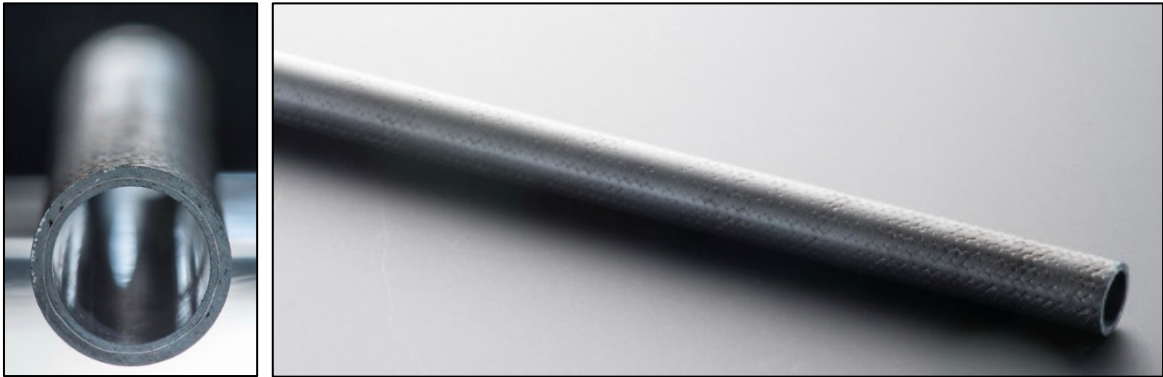
Figure 13.2. Segment of SiC/SiC fuel cladding including a metal liner
