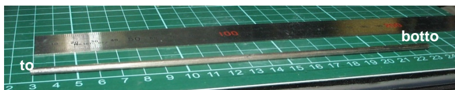
Figure 17.2. U-20 Pu-10 Zr fuel slug fabricated by injection casting method in a collaboration project between CRIEPI and JAEA
