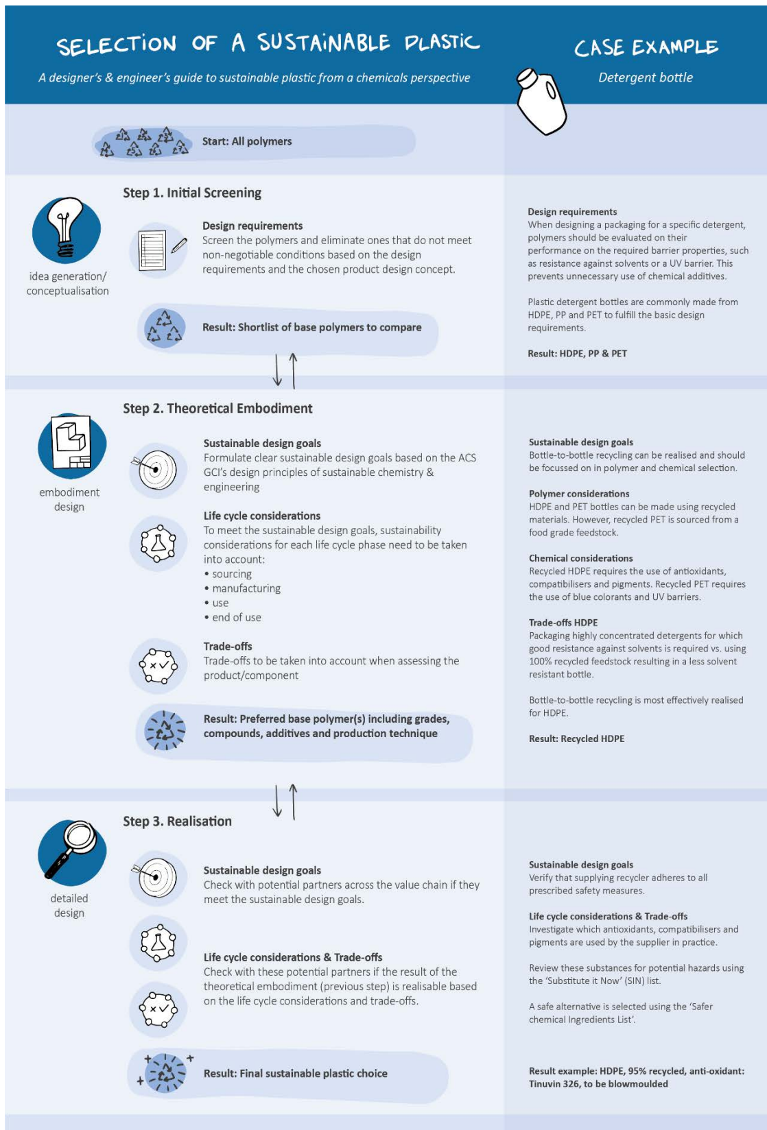
Figure 9.1. Main steps of the sustainable plastic selection process from a chemicals perspective and a case example
