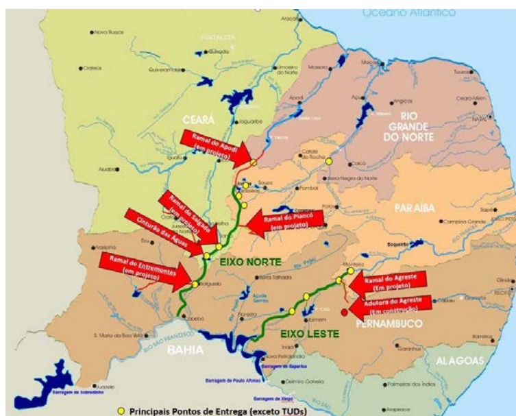
Figure 2.4. Northern and eastern routes of the São Francisco water transfer project
