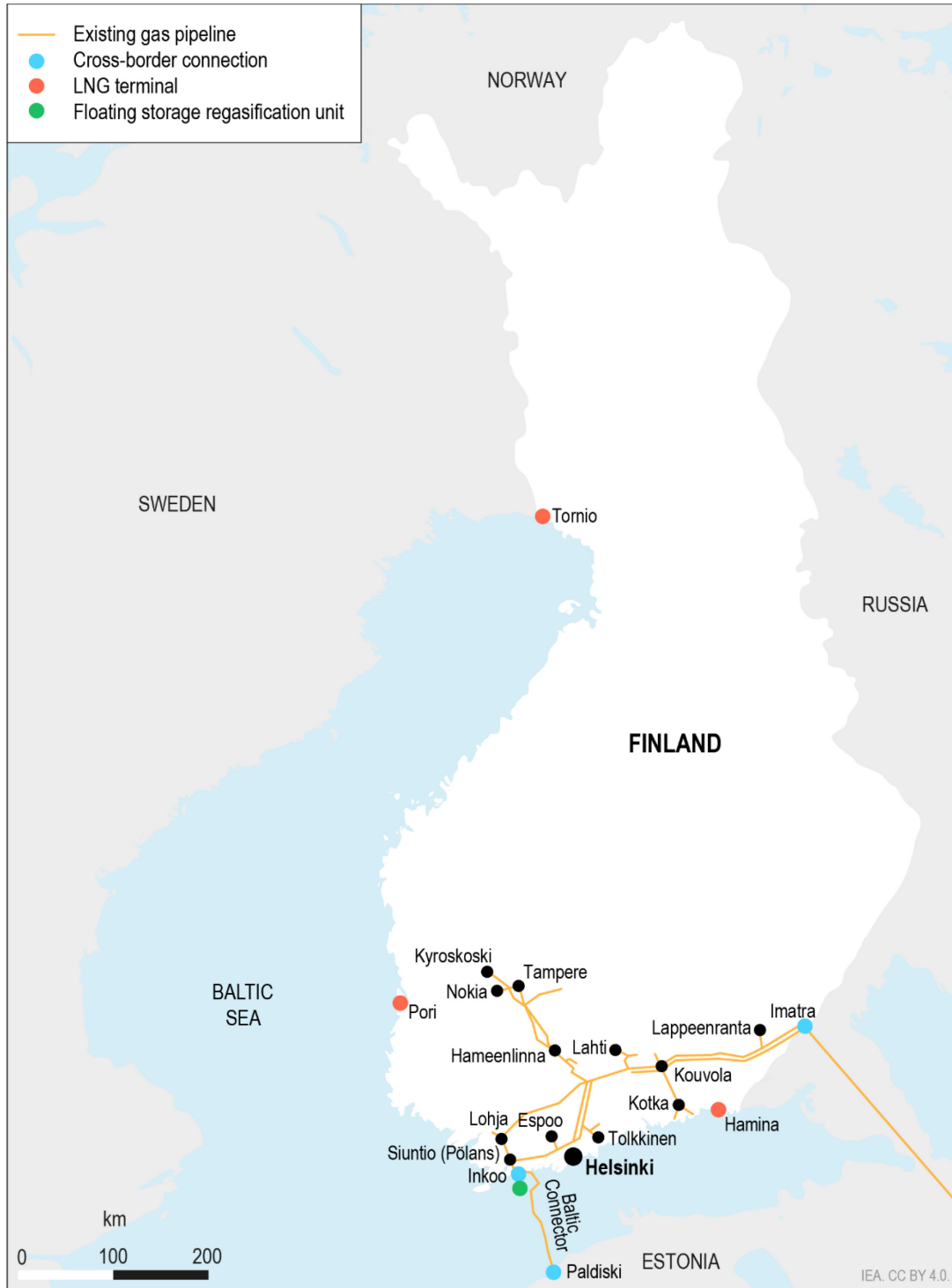
Figure 8.4 Finland's natural gas infrastructure
