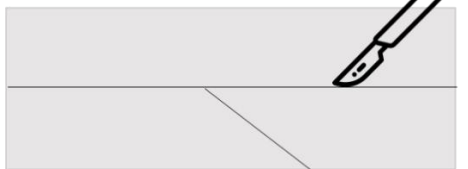
a. Collector (modified microscope glass slide)
