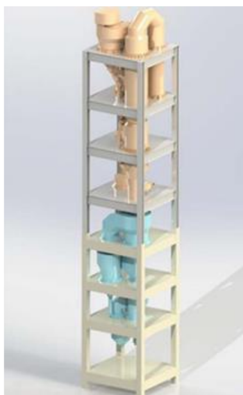
Figure 4.3. Flash clay calciner tower – 3d-render
