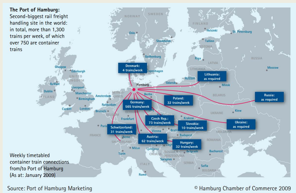
Figure 1.14. Container train connections with Hamburg's port
