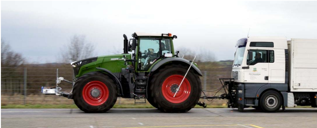
Figure 8: Specific truck for the compulsory drawbar test
