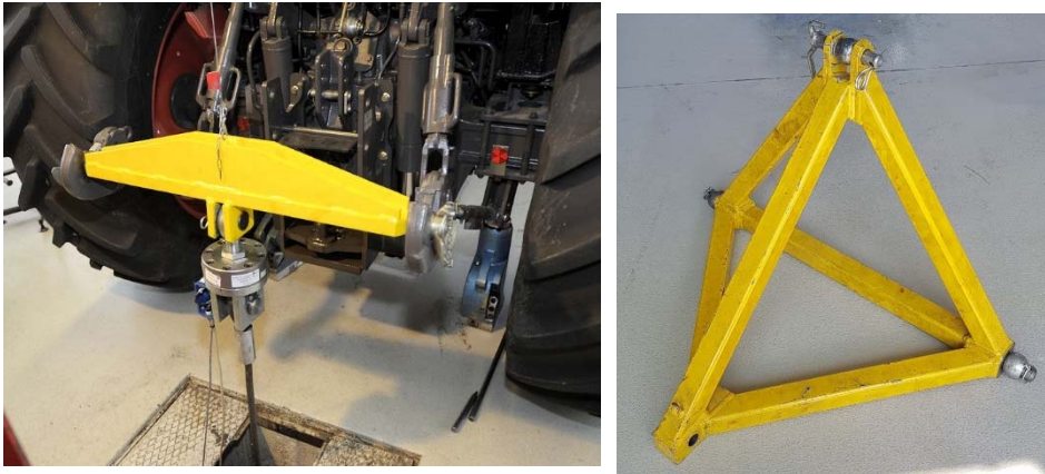
Figure 7: Composition for hydraulic lift measurement at the lower hitch points (l.). Frame for lower and upper links (r.)
