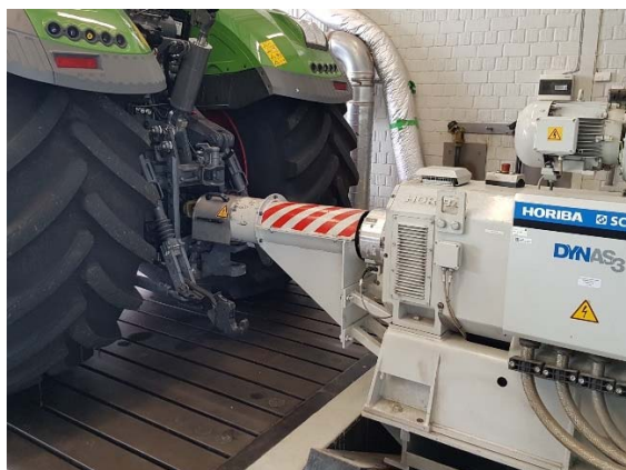
Figure 5: Dynamometer for Power-Take-Off (P.T.O.) measurements
