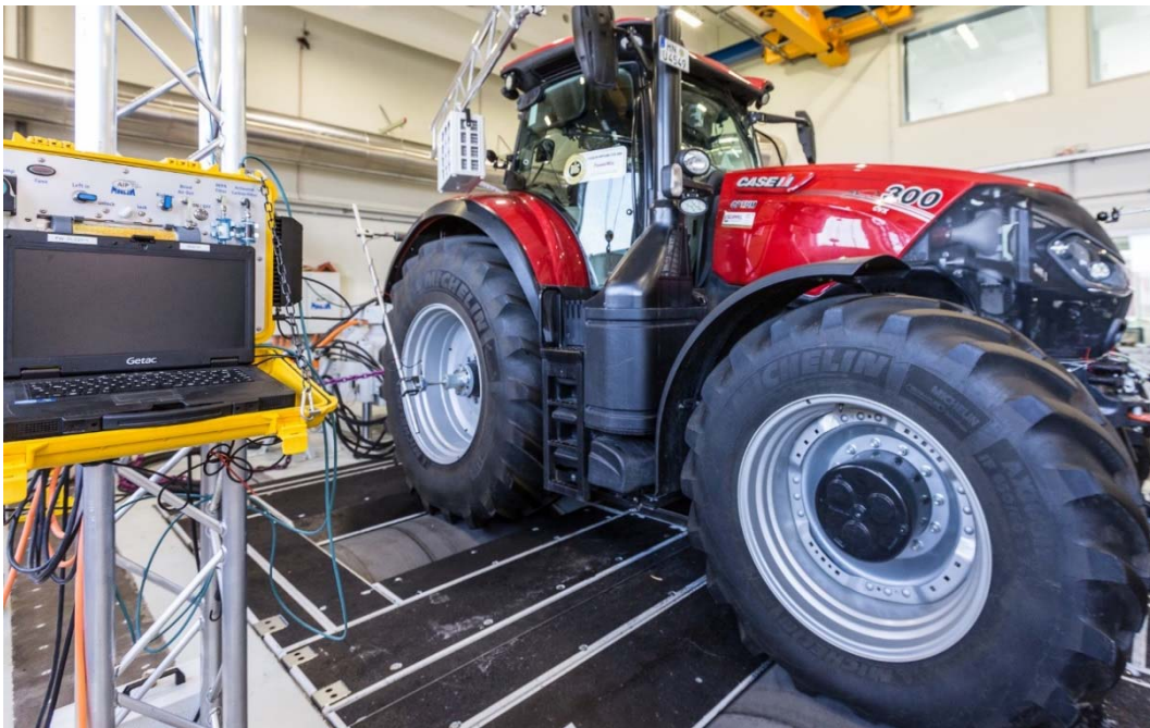
Figure 9: Chassis dynamometer for drawbar measurements
