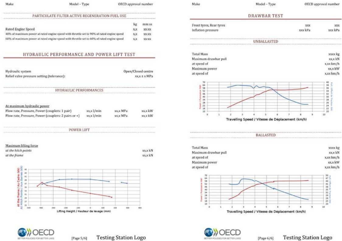
Figure 16: Pages 5 and 6 of an OECD Code 2 abstract: hydraulic-, powerlift, and drawbar test results
